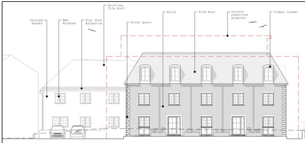
Fig.8 Proposed extension frontage elevation (original scheme shown dotted)
